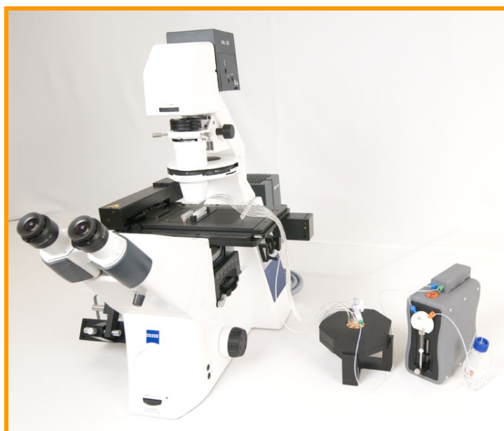
Mirus™ Evo Nanopump and MultiFlow8 connected to Vena8 biochip on inverted microscope
